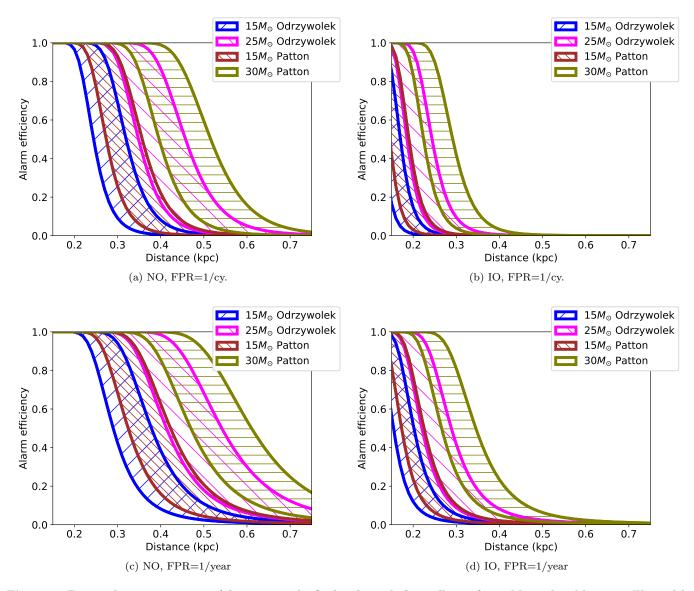
Figure 9. Expected maximum range of detection in the final 12 hours before collapse, for 15 M<sub> $\odot$ </sub> and 25 M<sub> $\odot$ </sub> stars. The width of the bands shows uncertainty due to levels of background in SK-Gd, and the difference between models of  $\gamma$ -ray emission from TNC on Gd.
