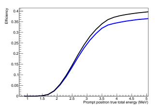
Figure 8. Trigger and selection efficiency for DC events against prompt positron true total energy. Above 4 MeV positrons are efficiently triggered and reconstructed, and so the efficiency is determined by the triggering and selection of the delayed part of the event. The result with the alternative Gd  $\gamma$ -ray-cascade model is shown in blue.
