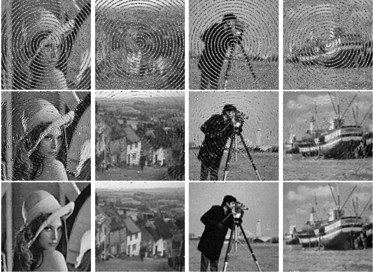
Figure 5.5: The restored results of images blurred by fspecial('disk',3) and corrupted by random-valued impulse noise (level s = 36.83\% ) at specific set and Gaussian noise (STD \sigma = 5 ). Top row: blurry and noisy images; Middle row: the results restored by Fast_IFASDA; Bottom row: the results restored Ada_Fast_IFASDA.
