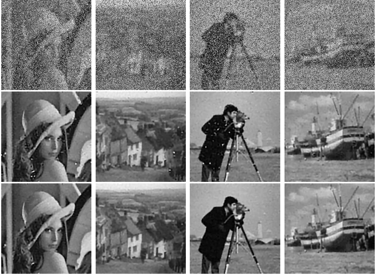
Figure 5.4: The restored results of images blurred by fspecial('disk',3) and corrupted by random-valued impulse noise (level s = 55\% ) at random set and Gaussian noise (STD \sigma = 5 ). Top row: blurry and noisy images; Middle row: the results restored by Fast_IFASDA; Bottom row: the results restored Ada_Fast_IFASDA.
