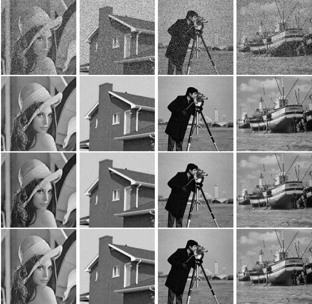
Figure 5.2: Denoising results of images contaminated by both Gaussian noise and salt-and-pepper impulse noise with \sigma = 10 and s = 30\% . Top row: noisy images; Second row: the results restored by AMF; Third row: the results restored by TVL1; Bottom row: the results restored by total variation blind inpainting using AOP.
