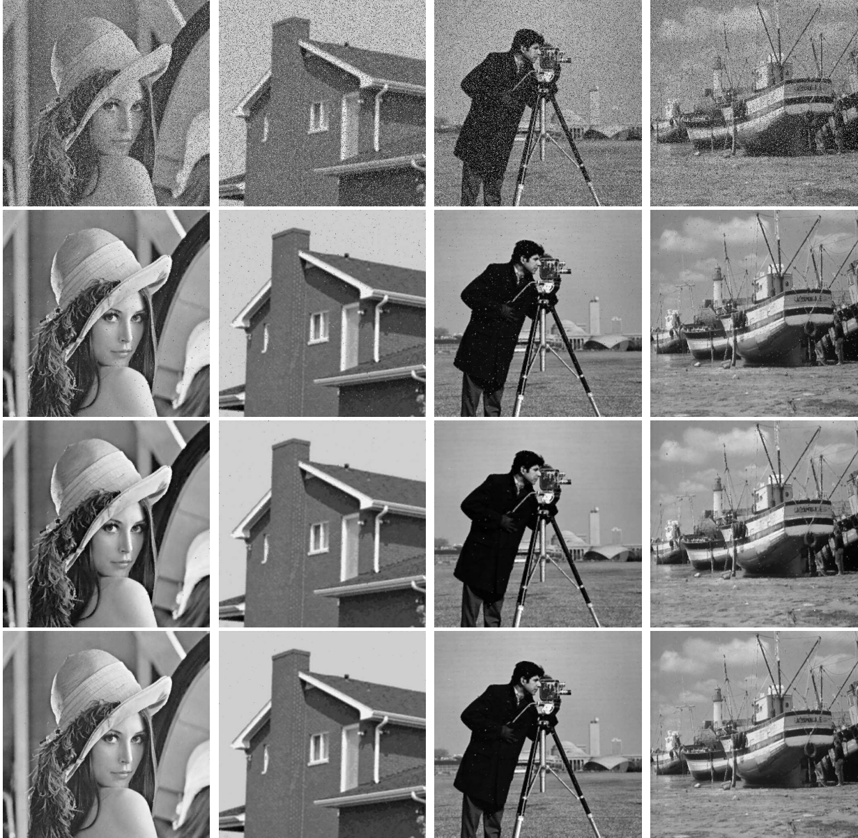
Figure 5.3: Denoising results of images contaminated by both Gaussian noise and random-valued impulse noise with \sigma = 10 and s = 25\% . Top row: noisy images; Second row: the results restored by ACWMF; Third row: the results restored by TVL1; Bottom row: the results restored by total variation blind inpainting using AOP.
