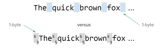
The byte overhead of per-token headers is made up for in most cases by the freedom to forgo most delimiters and whitespace characters that would normally be necessary between tokens. In the case of strings less than 15 bytes long, the single-byte preamble overhead is exactly equivalent to that of a C-style string with a trailing zero-byte terminator, but Infra strings are unambiguous to parse or skip because the length is known up front.
