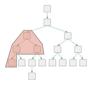
Each Patch execution context has one of these overlays. The overlay is empty until the first edit operation occurs. With each successive edit, or navigation after an edit, it expands just enough to include that location. Any value that is already part of the overlay can be mutated over and over with amortized cost, such as when inserting and removing a series of items in a list.
