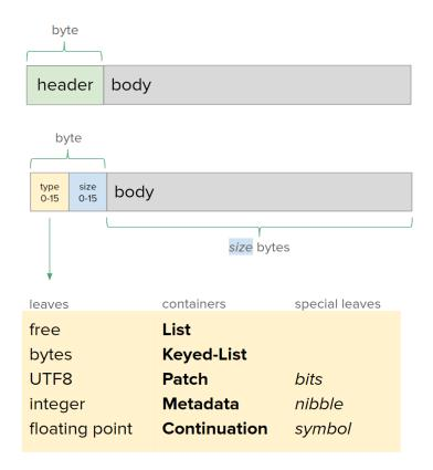
Body length 15 is reserved to signal a multi-byte header mode where the length is instead encoded using a variable length unsigned integer encoding. We find Dluglosz' encoding [21] to be efficient and well designed for this purpose. This is the encoding used for VLIs in the ZIP2 format. type
