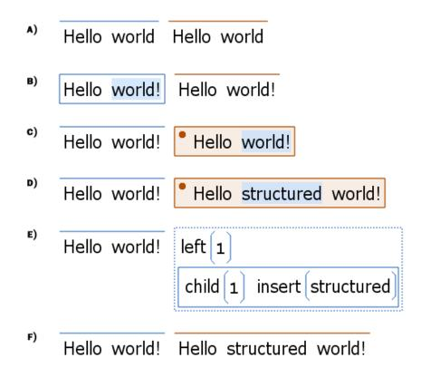
Edit Capture When a direct edit is attempted in the UI, the edit event is passed up the tree. If it makes it out the top of the root node, the edit event is applied. If the event encounters a Patch that is in 'record mode', the edit will be transformed before it continues on its way up the tree. The transformation is a conversion from a direct edit, to the appending of Patch code.
