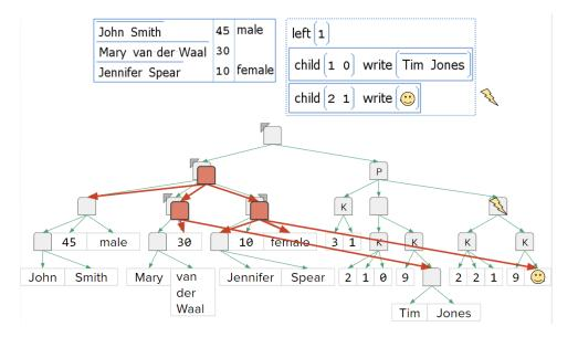
When this write occurs, no additional cloning need occur since the parent being changed is already part of the overlay.
