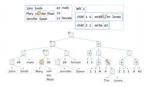
At this point, the Patch execution is at a write instruction. This will cause the parent to be cloned, since it is not already.
