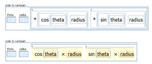
The top row shows the Patch tree without any evaluation, and the bottom row is the reduced (semi-evaluated) form that would appear in the editor (see the discussion on Native-Service Objects for clarification). The pale blue boxes labeled 'theta' and 'radius' are *Parameter* symbol elements, which are meant to be used as placeholders for a future value - perfect to play to role of an input parameter.
