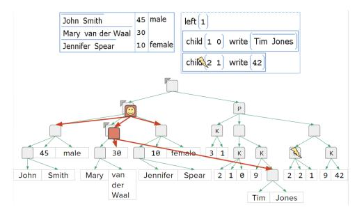
Since the last two statements were nested, and the end of the inner list has been reached in the execution, the cursor is 'popped' back to were it was when that list started. This has caused an additional node to be cloned so that the cursor does not end up outside of the cloned region.
