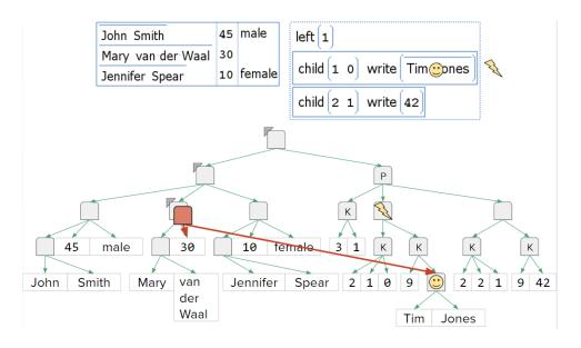
After the write, this virtual tree is technically a directed-acyclic graph because the value written is only referenced from its place in the Patch code.
