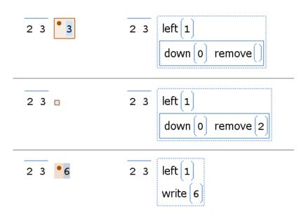
Note that the refactoring engine is attempting to keep the code simple by catching opportunities to merge or eliminate statements. The second 'remove' was able to be merged in with the first, and ultimately the 'remove' commands are rendered irrelevant by a write that replaces their root.
