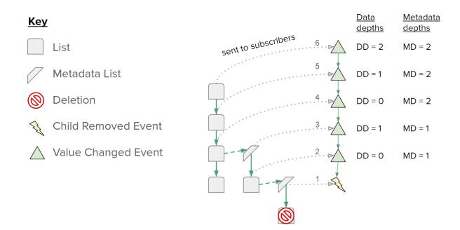
A Patch execution can build higher-level observers out of combinations of subscriptions to these basic events. We call these higher-level observers monitors. We identify six classes of monitor that precisely cover the conditions that can cause a change in Patch result.
