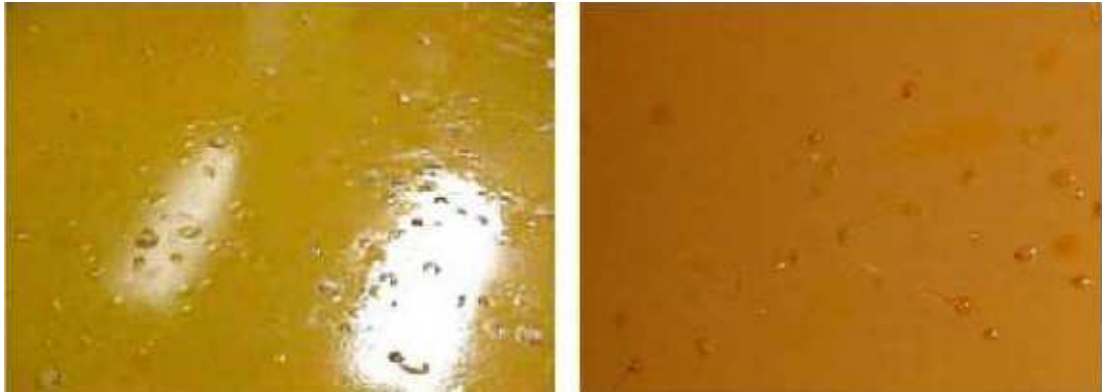
Figure 2.21: Photographs of linseed oil coating defects for high temperatures; cause of RPC degradation.
