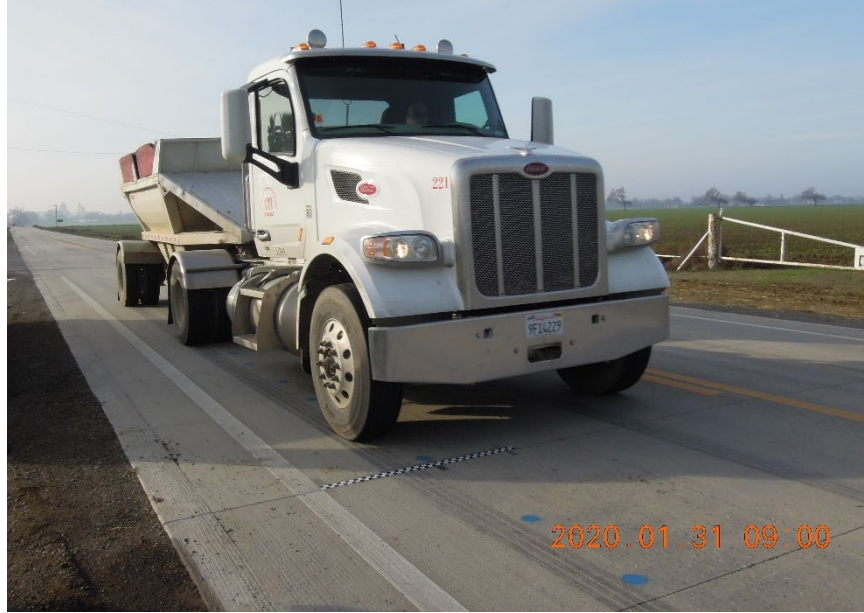
Figure 8.20: Experiment truck passing over instrumented slab (IP A21).
