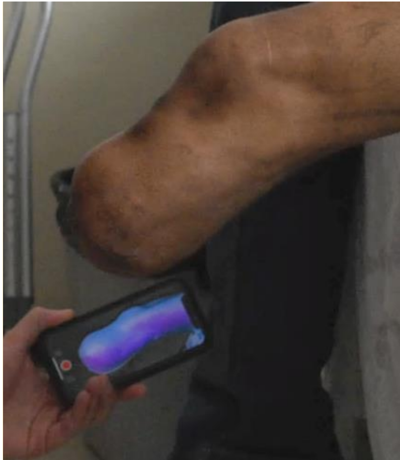
Figure 6.4. A smartphone is used to 3D scan an amputee's limbs using the front-facing TrueDepth camera on the iPhone.
