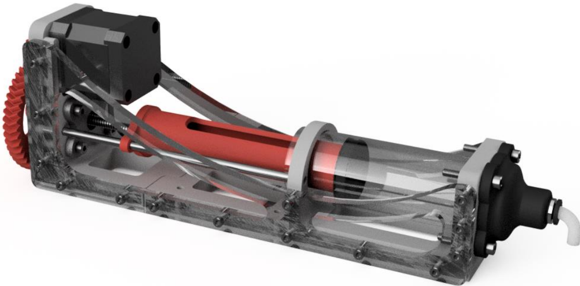
Figure 3.3. The feed system was designed and rendered in Fusion 360. This feed system unit has a capacity of 100 cc, provides excellent positional precision using a geared down leadscrew, and can generate pressures over 100 psi.
