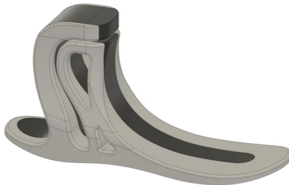
Figure 6.21. Multi-material printing enables to fabrication of the ankle-foot complex with tailored load-displacement response and energy return. Carbon fiber filled nylon is stiffer and springier than unfilled nylon, and the spatial tailoring of each material will enable enhanced functionality.
