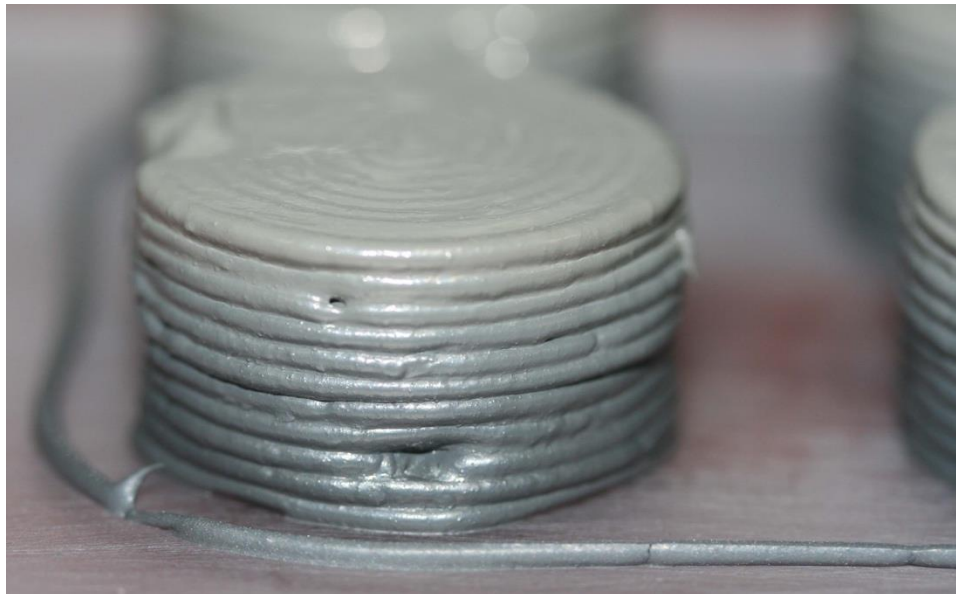
Figure 3.12. Gradient boron carbide (bottom) to silicon carbide (top) 1-inch diameter cylinder produced by DIW. Print parameters are: 1.2-mm layer height, 1.2-mm nozzle width, 4-mm/s print head speed, and center-to-perimeter concentric fill pattern.
