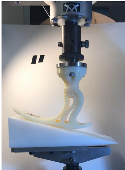
Figure 6.11. Mechanical testing of the 3D printed prosthetic feet (unfilled nylon) was achieved using angled HDPE blocks, 15 degrees for toe loading and 20 degrees for heel loading, on an Instron 3367 Universal Testing System.
