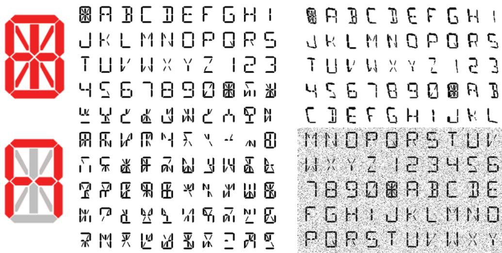
Figure 45: *left*) The 14-segment template used to create characters. We can turn on/off each segment independently to generate a vast alphabet. *middle*) An example of a page which is generated from the process. *right*) A page of the book after adding polynomial distortion (*top half*), and Gaussian noise with mean 0 and variance 0.10 (*bottom half*)
