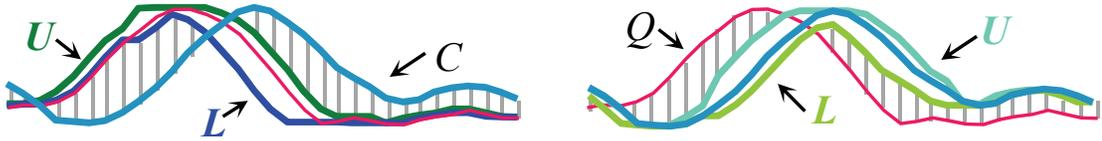
Figure 8: *left*) Normally the  $LB_{Keogh}$  envelope is built around the query (see also Figure 4.*right*), and the distance between  $C$  and the closer of  $\{U,L\}$  acts as a lower bound. *right*) However, we can reverse the roles such that the envelope is built around  $C$  and the distance between  $Q$  and the closer of  $\{U,L\}$  is the lower bound
