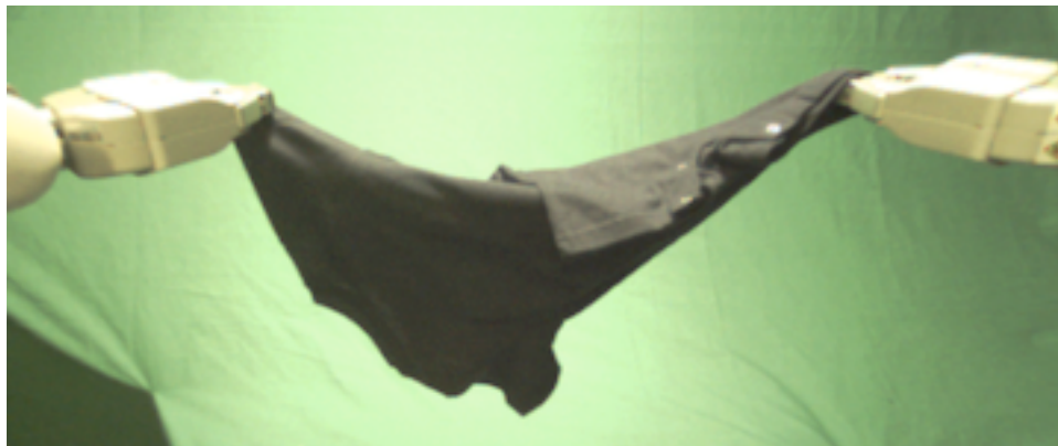
Figure 3.9: A cloth configuration in which the article is flipped over itself and therefore not in the minimum-energy configuration predicted by our simulator.
