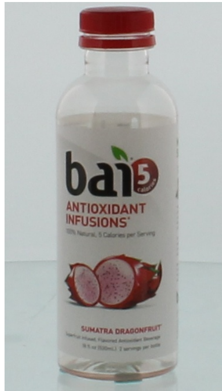
Figure 4.8: An example object for which Kinect-style RGB-D sensors yield poor-quality point clouds.
