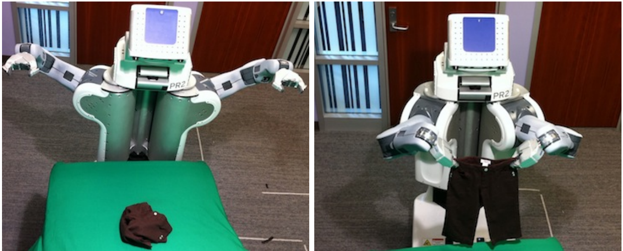
Figure 3.1: The PR2 starts with a pair of pants in a crumpled initial configuration, and then manipulates the pants into the desired configuration.
