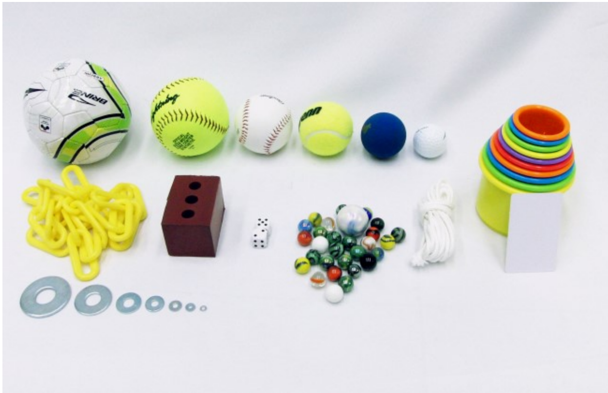
Figure 5.4: Shape items included the YCB Object Set. Back: mini soccer ball, softball, baseball, tennis ball, racquetball, golf ball. Front: plastic chain, washers (seven sizes), foam brick, dice, marbles, rope, stacking blocks (set of 10), blank credit card.
