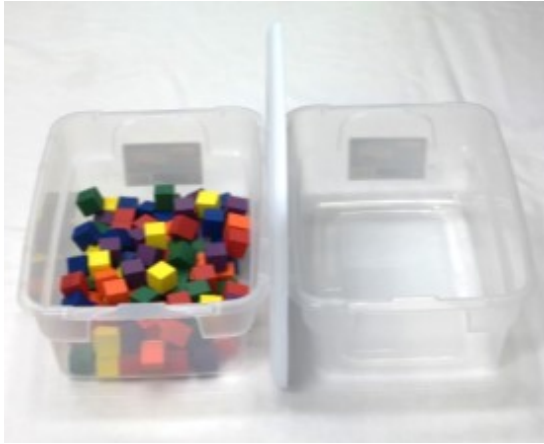
(a) Improved box-and-blocks test objects: set of 100 wooden cubes, two containers, and an obstacle (container lid) between them.
