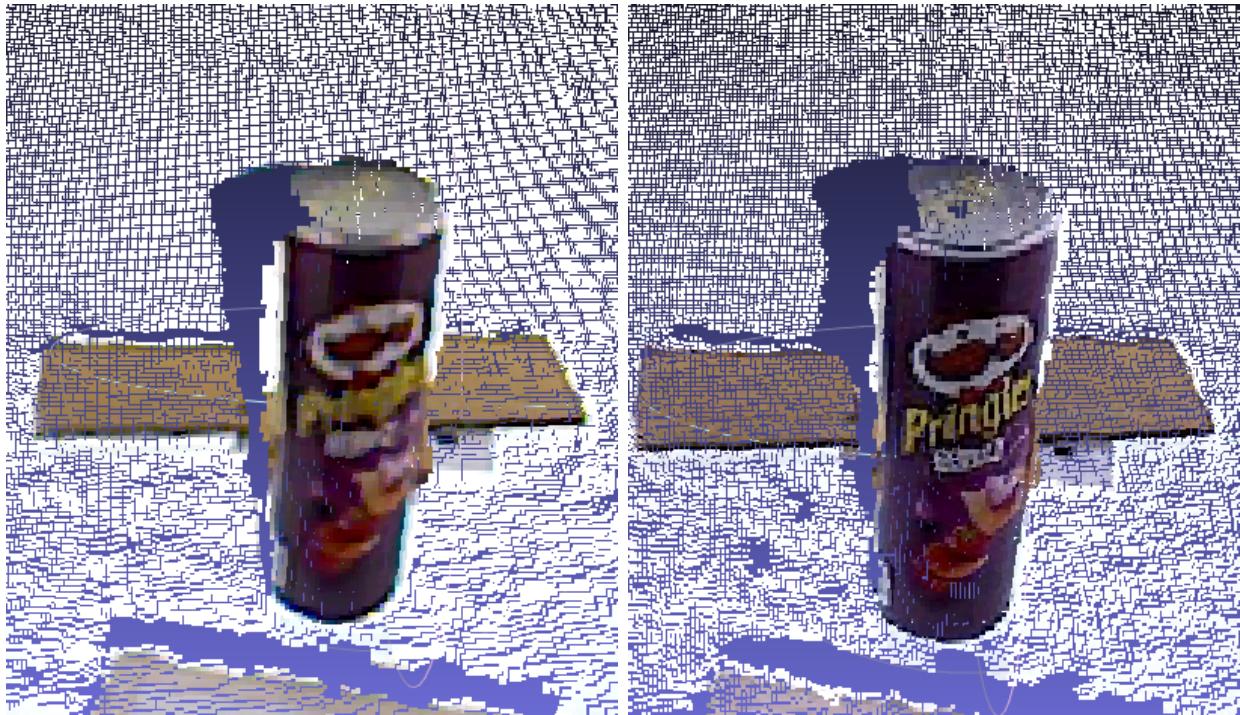
Figure 4.3: Comparison of hardware and software registration. The left image shows a hardware-registered point cloud. Note the bleeding of the cardboard in the background onto the Pringles can and the low resolution of the color data. The right image shows a software-registered point cloud using our calibration. Most of the bleeding of the cardboard onto the can has been fixed, and we can use higher-resolution color data.
