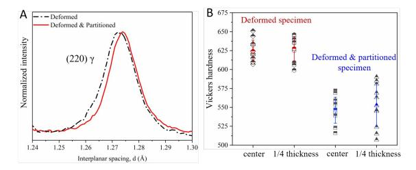
**Fig. S4.**(A) The neutron profiles of the deformed as well as the deformed and partitioned (D&P) specimens. (B) The Vickers hardness values of the deformed and D&P specimens measured at locations in the 1/2 (center) or 1/4 thickness to the surface.
