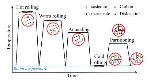
**Fig. S1.**Schematic illustration of the thermomechanical process used to produce the steel in this work.
