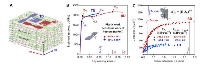
**Fig. 2. Tensile and fracture properties of the present steel.** (A) Schematic diagram describing the orientations of the dog-bone shaped tensile specimens and the compact-tension C(T) specimens relative to the thin-sheet steel. (B) Engineering stress-strain curves of the present steel deformed under tension along the RD and TD orientations. (C) The *J*-integral based resistance curves (*J*-R curves) measured from the C(T) specimens at room temperature.
