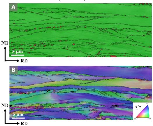
**Fig. S2.**Microstructure of the intercritical annealed specimen. (A) EBSD phase map. Green: austenite; Red: ferrite. (B) EBSD orientation map. High-angle grain boundaries (>15°) are marked by black lines.
