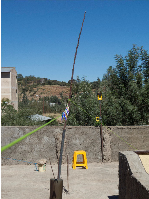
The GPS base-station on the roof of the dighouse in Indaselassie (December 2016); its corrected coordinates are: 37P / 421758.53 E / 1558870.18 N / 1913.79 mASL
