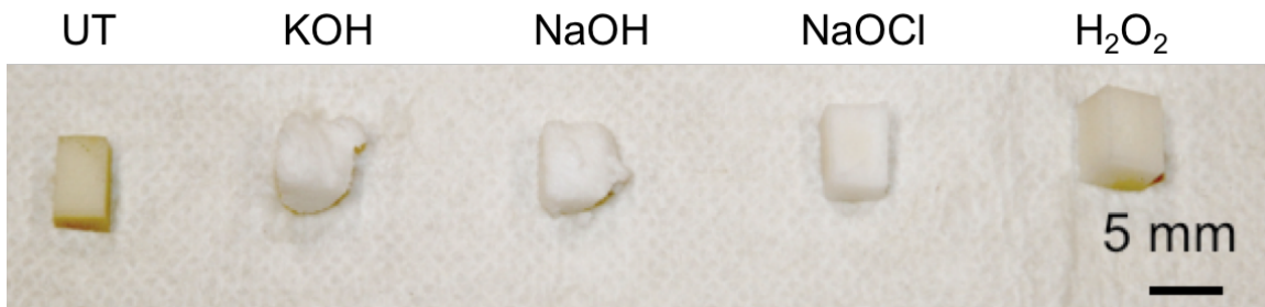
Figure 2.1. Photograph of untreated (UT) porcine femur sample and specimens after six days of treatments using KOH, NaOH, NaOCl, and H 2 O 2 .
