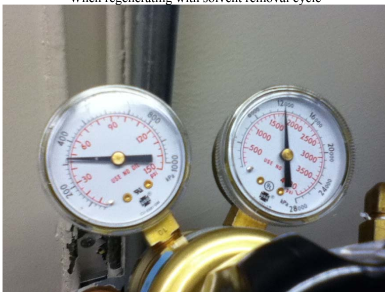
Check the regen gas cylinder that it has at least 400 psi (cylinder NI HY10-K from praxair)
