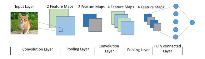
Figure 2.4: An example of a convolution neural network architecture.
