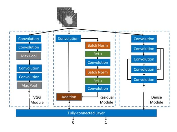
Figure 4.1: Framework of hybrid ensemble CNN model for lung nodule classification.
