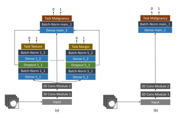
Figure 4.5: Framework comparison between proposed HSCNN and baseline 3D CNN. (a) proposed HSCNN architecture; (b) baseline 3D CNN architecture. Compared with the proposed HSCNN, baseline model has the same structure but without the low-level semantic task component.
