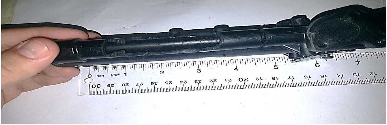
Figure 3-9: Heater internals, cut open to show after degradation in caused by contact with the oil Drakesol 260AT
