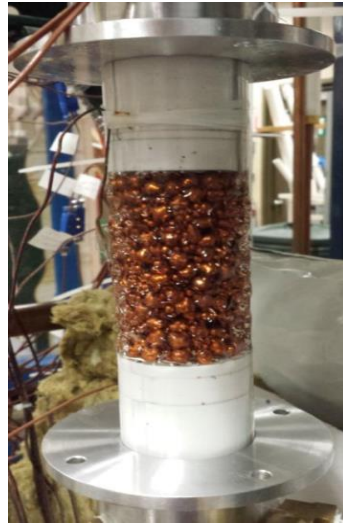
Figure 3-18: Left – Drill press used to get a press fit between the glass tube and the aluminum flanges. Right - Test section filled with copper pebbles for heat transfer coefficient measurement experiments
