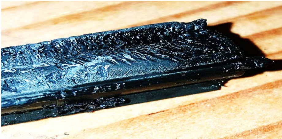
Figure 3-10: Close-up of material degradation from contact with medium-temperature oil
