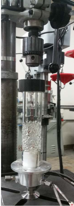
Figure 3-18: Left – Drill press used to get a press fit between the glass tube and the aluminum flanges. Right - Test section filled with copper pebbles for heat transfer coefficient measurement experiments
