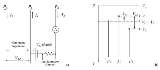
**Fig. 4** The equivalent circuit of triple probe with direct display system and its potentials: a) Equivalent circuit and b) Potentials of each probe tip.
