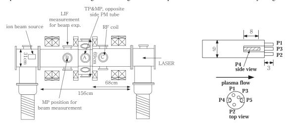
Fig. 1 Schematic diagram of the test facility and diagnostic systems
