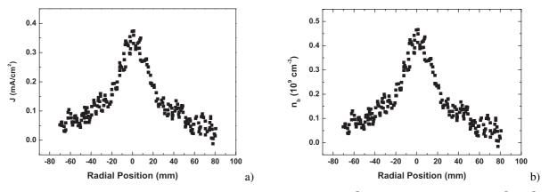
Fig. 3 The reference supersonic ion beam density: a) current density, J (mA/cm<sup>2</sup>) and b) number density,  $n_b$  (×10<sup>9</sup> cm<sup>-3</sup>) at 80 watt RF power input with f = 18.75 MHz and  $3 \times 10^{-4}$  Torr.
