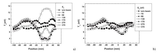
**Fig. 5** Electron Temperatures: a) from the conventional TP theory and b) from a new theory with compensation of supersonic ion beams.
