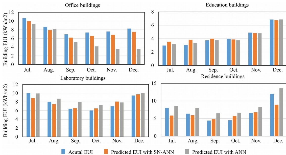
Fig. 9 The building EUI prediction results for the office, educational, laboratory and residential buildings.
