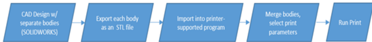
Figure 4: Workflow diagram from concept design through 3D print.
