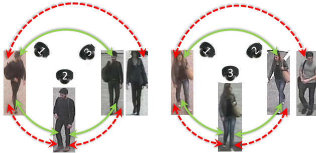
Figure 2.4: Two examples of correction of inconsistent re-identification from WARD dataset. The red dashed lines denote re-identifications performed on 3 camera pairs independently by FT method. The green solid lines show the re-identification results on application of NCCA on FT. The NCCA algorithm exploits the consistency requirement and makes the resultant re-identification across 3 cameras correct.
