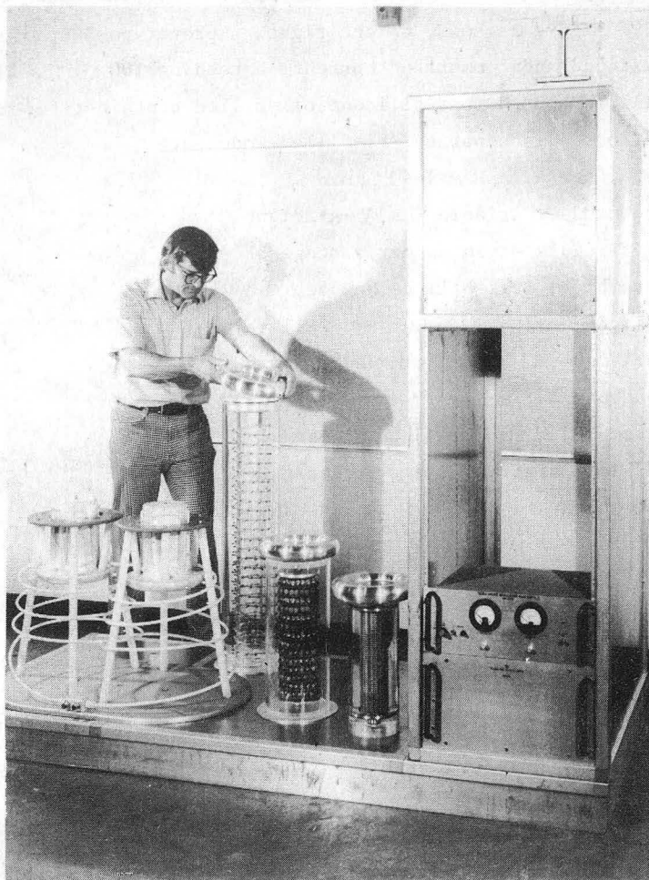
Figure 5. Shunt Regulator Cart and Related Components
