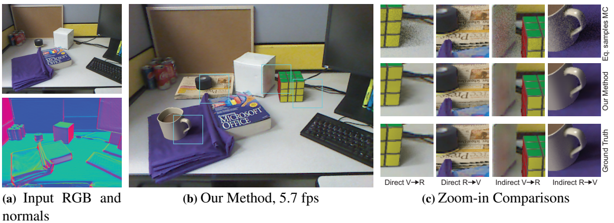
Figure 6.1: We start with a stream of RGBD images from a Kinect camera, and use SLAM to reconstruct the scene. (a) shows the input RGB image and reconstructed normals. In this DESK scene, we insert a virtual rubik's cube, a newspaper, and a coffee mug, as shown in (b) where environment illumination (both direct and 1-bounce indirect) are computed using Monte Carlo (MC) path tracing followed by filtering. The full system runs at 5.7 fps. We show comparisons of our result with unfiltered MC with equal samples, which is very noisy, and reference, which takes 60\times longer to render.
