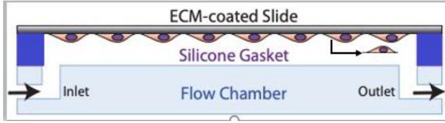
Figure 1: A: Schematic of parallel plate flow chamber.
