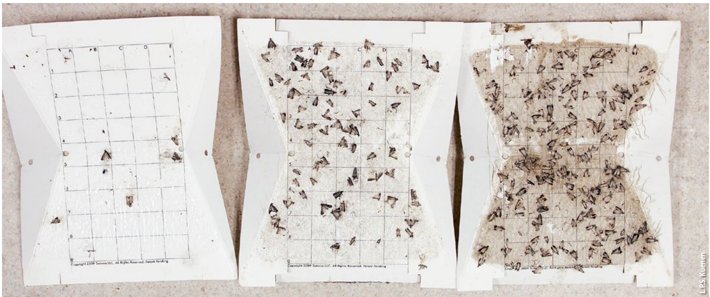
Fig. 1. Trap bottoms from Suterra wing traps containing 5 (left), 79 (middle) and 149 (right) NOW males. Note the fouling of glue surfaces with moth bodies and scales on the two higher-count traps. Saturation begins at approximately 50 moths.
