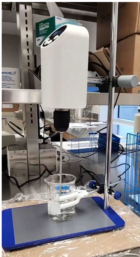
Figure 2.4.1 Mimicking a washing machine cycle using a tergotometer and beaker with water and detergent
