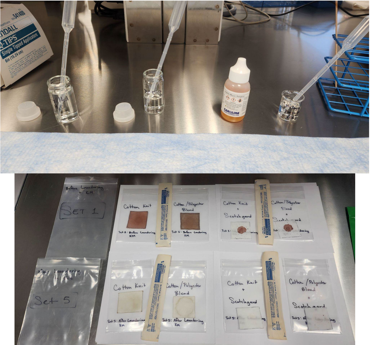
Figure 2.A Kastle-Meyer Test set-up. The reagent and procedure for completing the test is seen in the top photo listing the components needed to complete the test from left to right: distilled water, 70% ethanol, Kastle-Meyer Reagent from the Carolina Biological Supply Company, and 3% hydrogen peroxide. The bottom photo shows Sets 1 and 5 that will undergo the KM testing procedure and the necessary cotton swabs (two in a pack) that will be used for each sample.
