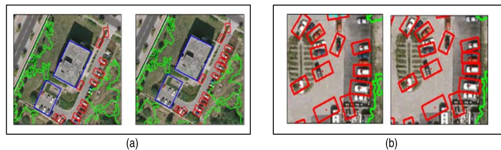
Fig. 22 Close up views of our improvement during top-down prediction. Additional cars are added to the rows due to the presence of other collinear cars
