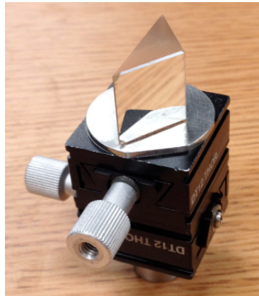
Figure 2.19: The custom prism showing one facet (15 x 9 mm) with the protective silver coating. The prism is used to direct the LGS beam to the DM and then back along the LGS beam's original path.
