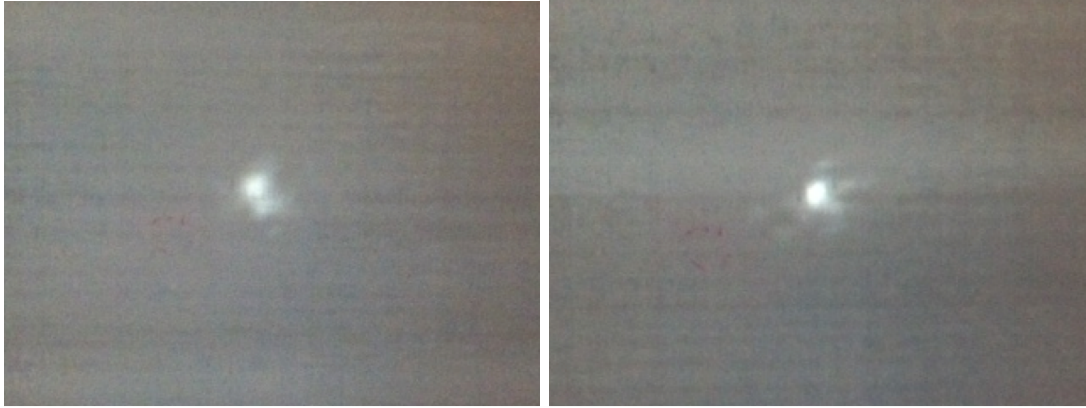
Figure 2.29: Left) Far-field profile of the sodium laser before optimization with the uplink DM. Right) Resulting far-field after optimization of 11 Zernike modes
