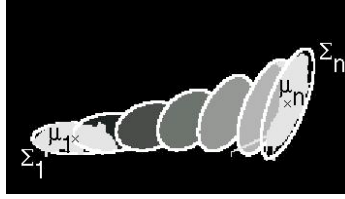
Figure 7.1: An example showing how the mean and covariance of the mouse on the left is linearly interpolated into the mean and covariance of the mouse on the right, using our algorithm for linear interpolation. The leftmost ellipse corresponds to (\boldsymbol{\mu}_1, \Sigma_1) and the rightmost ellipse corresponds to (\boldsymbol{\mu}_n, \Sigma_n) . The affine prior \hat{\mathbf{a}} transforms any of these ellipses to the ellipse on its right.
