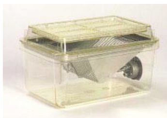
Figure 1.3: An image of a Static MicroIsolator cage common in research vivaria. Image taken from [2].
