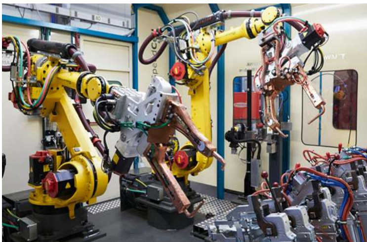
Figure 4.1: Industrial robots for spot welding
