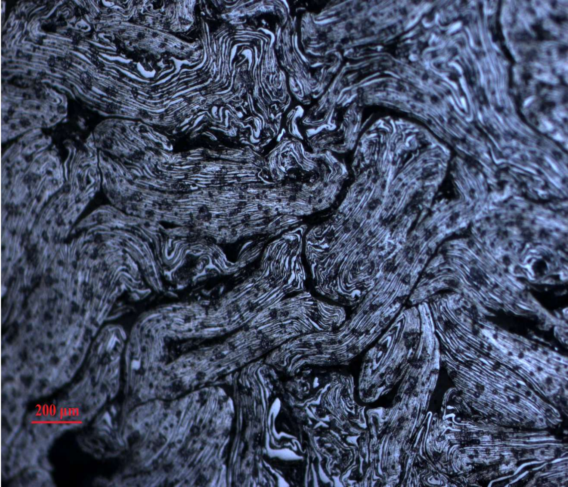
Figure 4.4: Microstructure of the 400 micron NiAl particles swaged with no core.
