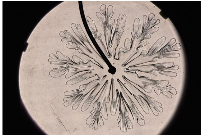
Figure 1.1. The formation of viscous fingers upon fluid displacement [29].
