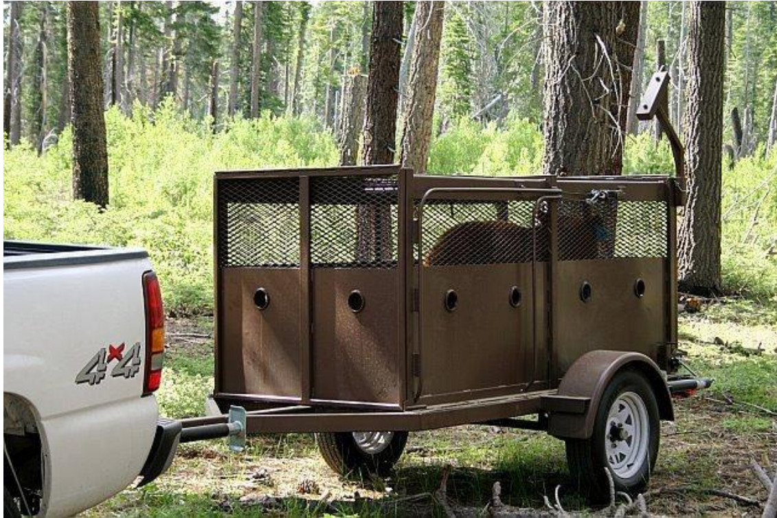
Figure 2: This figure shows box shaped trailer mounted bear trap, allowing for movement of bears to nearest possible habitat for release (Photo credit: Mario Klip).
