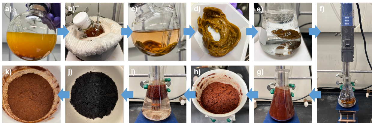
Figure 2.3. Step by step synthesis of FeOI-2. (a) Combined reactants in pressure flask. (b) Setup of flask in heating mantle. (c) Reaction end. (d) Rubbery solid resulting from the reaction. (e) Solid in ~ 250 mL DI water in 250 mL Erlenmeyer flask. (f) Tissue homogenizer inserted into flask. (g) Homogenization. (h) Product recovered after vacuum filtration. (i) Second homogenization (product floats to surface when not running homogenizer) (j) Dried 24 h in vacuum oven, then crushed with pestle. (k) Final product, FeOI-2, after additional 24 h in vacuum oven.
