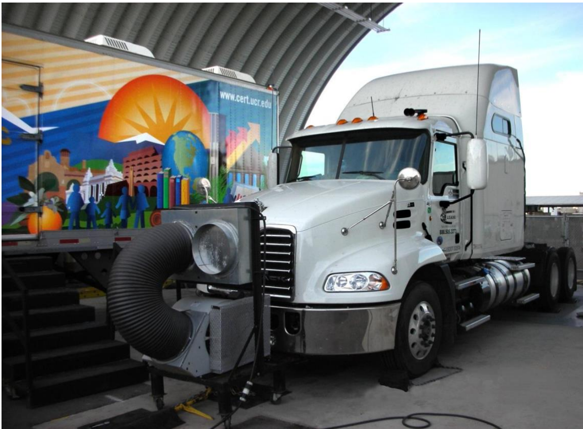
Figure 20. UCR's Heavy-Duty Chassis Dynamometer test facility
