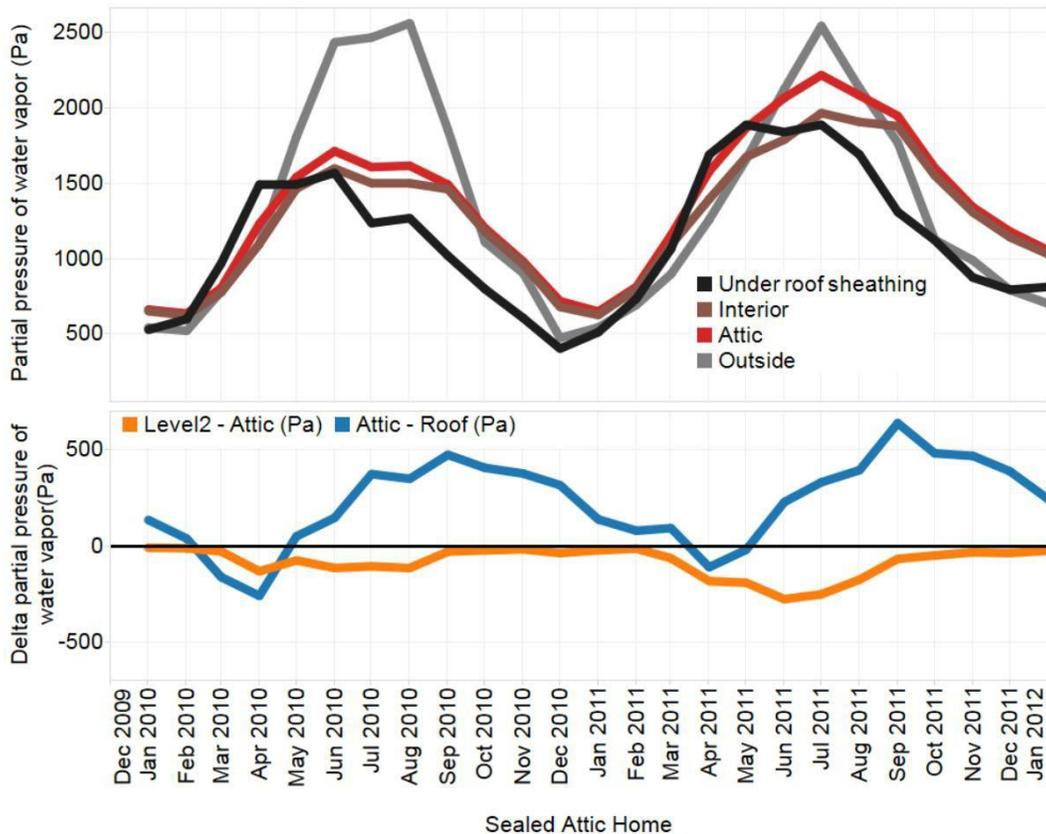
Figure 15 Monthly average partial pressures of water vapor in measurement locations in a sealed and insulated attic in a mixed humid climate. Source: Boudreaux et al. (2013).
