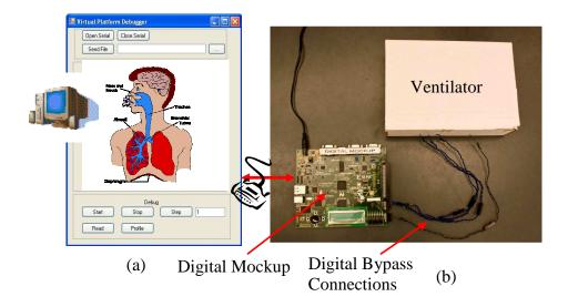
[Sirowy]. The rate at which the devices operate is user-defined by a separate PC-based debug interface, and shown in Figure 47(a).
