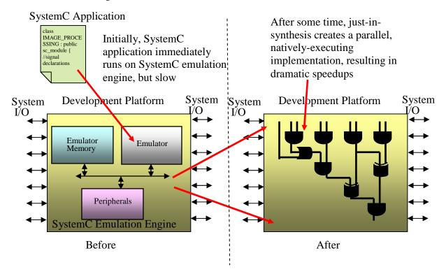
We introduce a transparent, server-side just-in-time synthesis framework to the SystemC-on-a-Chip framework that can override software emulation of SystemC applications and instead execute the application natively, yielding orders of magnitude speedups improvement over software emulation, and faster performance than native PC simulation. We demonstrate the usefulness of the framework by developing a full prototype for the Xilinx Virtex4 Ml403 development board using partial reconfiguration.
