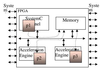
**Figure 27:** SystemC acceleration engines: **(a)** Internal structure. **(b)** Direct connection of two SystemC acceleration engines using a kernel bypass connection. In some situations, bypassing the bus and SystemC kernel can lead to significant performance benefits for a given SystemC description.
