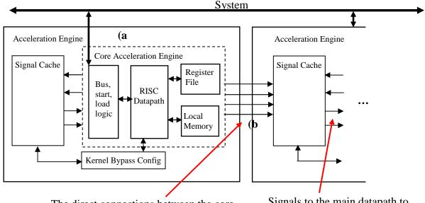
The direct connections between the core acceleration engine and the adjacent signal cache allow the two acceleration engines to communicate without using a shared bus memory
