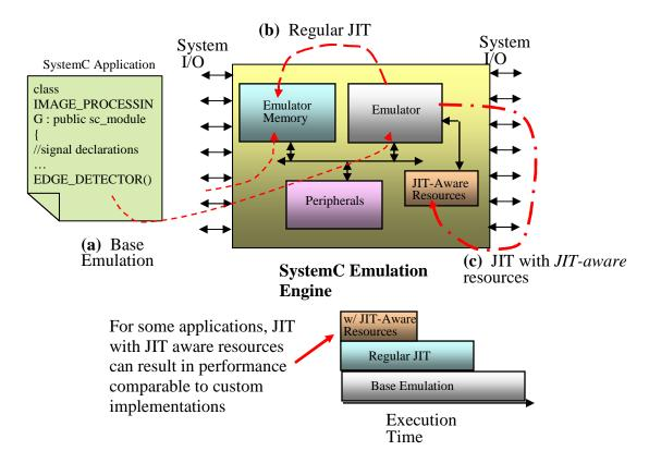
system performance to detect the new performance bottleneck. We could then change the processor architecture in order to alleviate that bottleneck, modify the JIT compilation accordingly, and repeat until no further improvements were found, as shown in Figure 31. The resulting JIT compilation, with the architecture containing JIT-aware resources as illustrated in Figure 16(c), showed substantial further speedups over the original JIT compilation.
