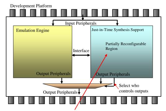
On initialization, just-in-time region is empty, and controls the mux to allow the emulation engine control of the output peripherals. After, the new bitstream changes the bit controlling the mux, giving the just-in-time region
