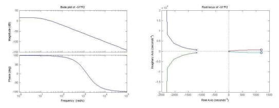
Figure 7.5 Bode (left) and root locus (right) plots of the plant, G1(s), combined with a second order Padé approximation of the delay introduced to the system by the BeagleBone Black's DAC.
