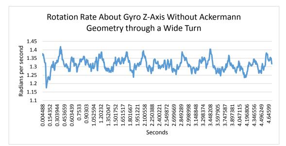
Figure 3.8: This plot shows the rotation rate about the z-axis of the gyroscope in radians per second through one full counterclockwise rotation of the vehicle without Ackermann geometry implemented. The motors were driven at 30% duty cycle as the vehicle traced out a circle of radius ≈0.481 m on a hard wood floor. This is a 51.2% wider turn than depicted in Figures 3-5 and 3-6. The comparison of Figures 3-7 and 3-8 shows similar results as that of Figures 3-5 and 3-6.
