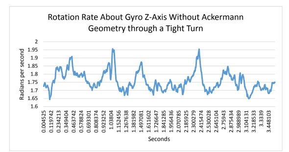
Figure 3.6: This plot shows the rotation rate about the z-axis of the gyroscope in radians per second through one full counterclockwise rotation of the vehicle without Ackermann geometry implemented. The motors were driven at 30% duty cycle as the vehicle traced out a circle of radius ≈0.318 m on a hard wood floor.
