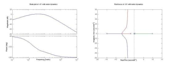
Figure 7.7: Bode (left) and root locus (right) plots of the plant G1(s) incorporating motor dynamics.
