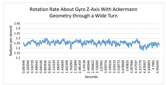
Figure 3.7: This plot shows the rotation rate about the z-axis of the gyroscope in radians per second through one full counterclockwise rotation of the vehicle with Ackermann geometry implemented. The motors were driven at 30% duty cycle as the vehicle traced out a circle of radius ≈0.481 m on a hard wood floor. This is a 51.2% wider turn than depicted in figures 3-5 and 3-6.
