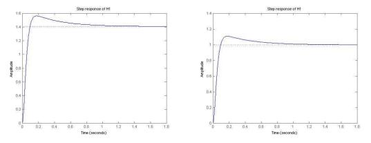
Figure 7.11: Step response of closed loop system without a loop prefactor on the left and with a loop prefactor on the right. Addition of the loop prefactor causes the response to settle at one as desired.
