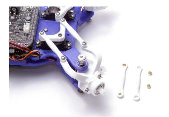
Figure 3.1: Close up of four bar steering mechanism.
