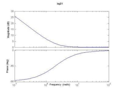
Figure 7.8: Bode plot of lag controller D\_lag (s).
