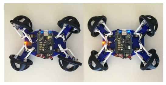
Figure 3.10: BeagleRover pictured in Lane Change drive mode on the left and Spin drive mode on the right.
