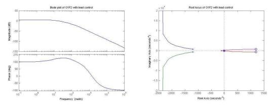
Figure 7.6: Bode (left) and root locus (right) plots of the plant, G1(s), and n=2 Padé approximation of the delay function, P(S), with lead control applied.
