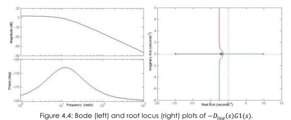
[50]. The Bode and root locus plots of the plant with negative gain and lag control combined are given in Figure 4.4.
