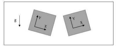
Figure 5.3: 2D representation of the axes of an accelerometer as it changes position in space. On the left hand side the x-axis reads slightly positive and on the right hand side the x-axis reads slightly negative.
