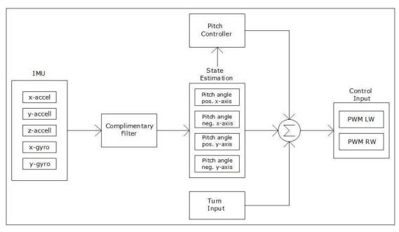
Figure 5.2: Software architecture of the balance function. PWM LW stands for PWM input to the left wheel and PWM RW is PWM input to the right wheel.
