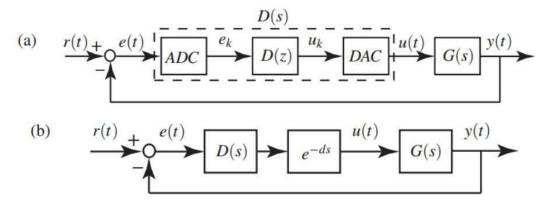
Figure 7.4: Block diagram of the controller/plant system. The bottom diagram shows the series connection of the controller and plant with the delay that arises from the digitalto-analog conversion of the discrete time controller output. The top diagram shows the discrete time version of the controller including the necessary data conversion for communicating with the sensors and motors.
