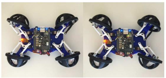
Figure 3.2: BeagleRover showing out of phase alignment of the wheels on the left and in phase alignment on the right. In the left image, the front wheels are rotated clockwise while the rear wheels are rotated counterclockwise. This is opposed to the right image where all wheels are rotated clockwise.
