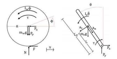
Figure 7.2: Free body diagrams of the wheel and rod.
