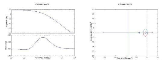
Figure 7.10: Bode (left) and root locus (right) plots of lead and lag control applied to the plant, G1(s), showing high gain at low frequencies for good tracking of the reference signal and ample phase bump at the crossover frequency.
