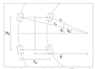
Figure 3.3: Ackermann steering geometry showing difference in radii between the circle traced by the inner wheel and the circle traced by the outer wheel in a right hand turn.
