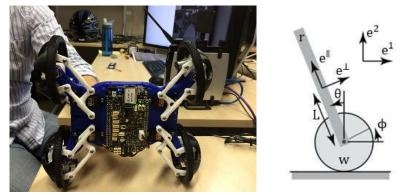
Figure 7.1: BeagleRover pictured on the left and 2D model of BeagleRover as a mobile inverted pendulum on the right.
