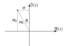
Figure 7.3: Graphical depiction of the s-plane showing how the natural frequency of the system is affected by pole location.
