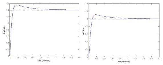
Figure 4.6: Closed loop step response of system without a loop prefactor on the left and with a loop prefactor of 1/1.4 on the right. The addition of the loop prefactor causes the step response to settle at one as desired.
