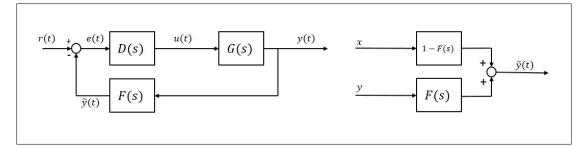
Figure 5.4: The block diagram on the left hand side illustrates integration of the complementary filter into the complete feedback system. Note disturbances and noise are not shown here. On the right hand side the block diagram of the filter itself is shown, where x and y in this case are the inputs to the low-pass and high-pass filters. Note the output of the filter is  $\tilde{y}(t)$  because no filter is ideal and y(t) will not be reconstructed exactly.
