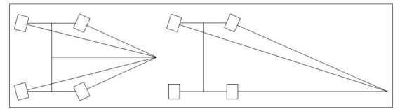
Figure 3.4: Comparing minimum turn radii of four wheel steering (left) vs. front wheel steering (right) on the same vehicle. Consider the front inner wheel in each drawing to be turned the maximum number of degrees as limited by the mechanical design. In the case of BeagleRover the maximum turn of the inner wheels is 17.5° before contact is made with the chassis.
