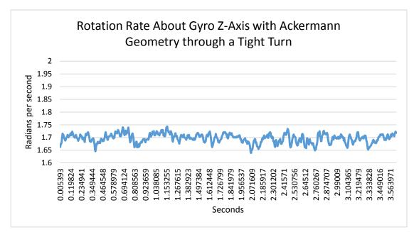
Figure 3.5: This plot shows the rotation rate about the z-axis of the gyroscope in radians per second through one full counterclockwise rotation of the vehicle with Ackermann geometry implemented. The motors were driven at 30% duty cycle as the vehicle traced out a circle of radius ≈0.318 m on a hard wood floor.
