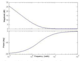
Figure 4.3: Bode plot of lag controller  $D_{lag}(s)$ .
