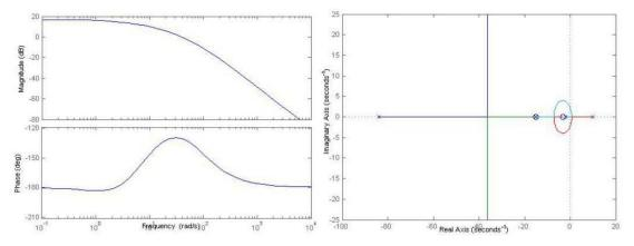
Figure 4.5: Final open loop Bode (left) and root locus (right) plots with lead and lag control where  $D_{lag}(s) = (s + 15)/(s + 86.4)$ .
