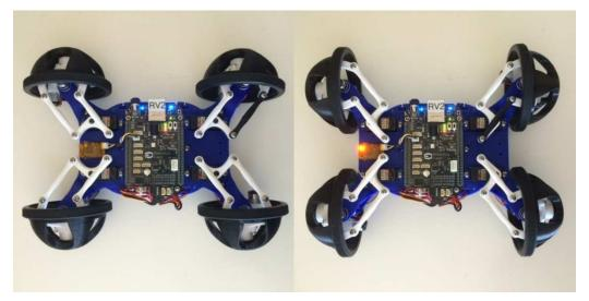
Figure 3.9: BeagleRover pictured in its Normal drive mode on the left and Crab drive mode on the right.
