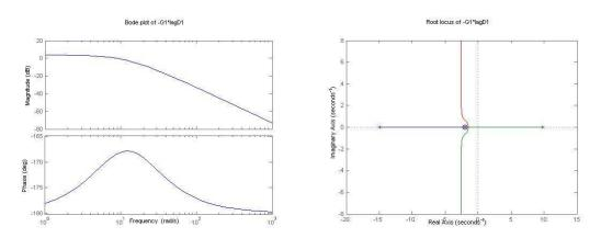
Figure 7.9: Bode (left) and root locus (right) plots of lag control combined with the plant G1(s).
