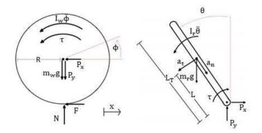
Figure 4.1: Free body diagrams of the wheel and rod.
