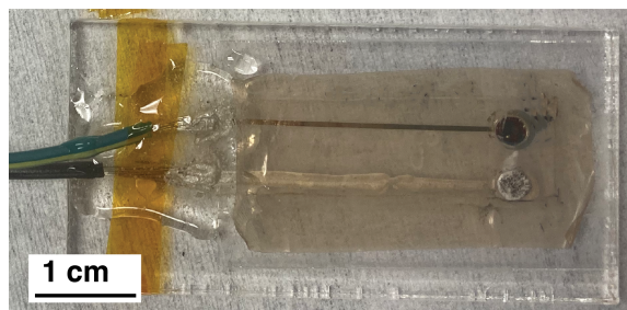
Figure 4.5: Picture of the assembled nitrate sensor. The nitrate sensor electrodes were adhered to an acrylic stake for mechanical support and ease of handling in experiments.
