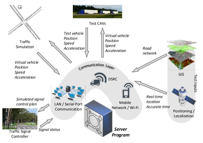
Figure 1. Components and data flow of the current HIL test tool
