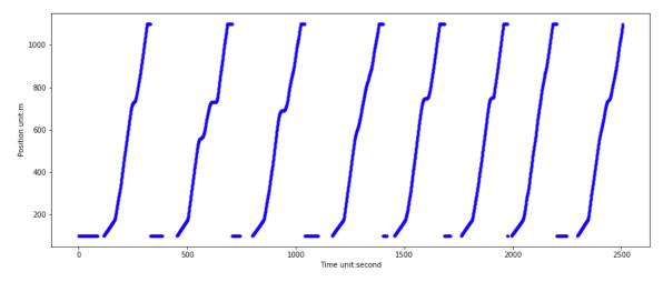
Figure 26. Aggregated Time-Space Diagram of Truck\_1 in Test #1
