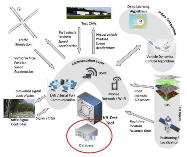
Figure 2. Test systems and data flow of the proposed HIL test tool
