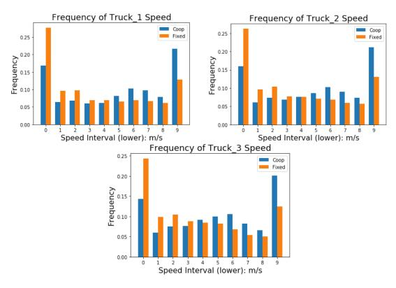
Figure 29. Comparison of truck's speed in different tests
