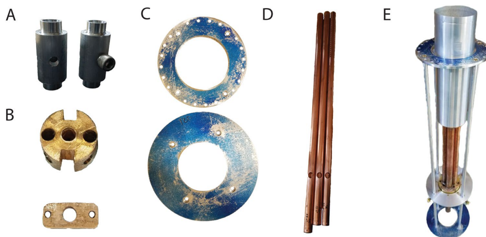
Figure 1.4: Hand-machined switched-angle spinning probe parts. A) Stand anchors, B) Proton-channel inductive stub and match plate, C) Top and bottom plates, D) Outer ground planes for ^1\text{H}/^2\text{H}/^{13}\text{C} tuning tube assemblies, E) Skeletal assembly of the SAS probe.
