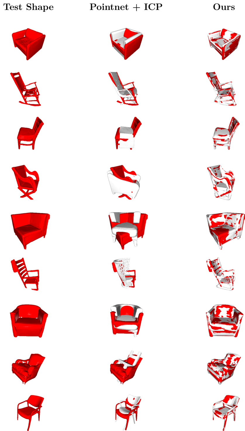
Figure B.2: Additional qualitative result on Redwood dataset. Left to Right, test shape, results using PointNet [81] and ICP, our proposed method. We have shown each method's result in gray overlaid with the input mesh in red. Our algorithm provides significant qualitative improvement on par with those displayed in chapter 4.
