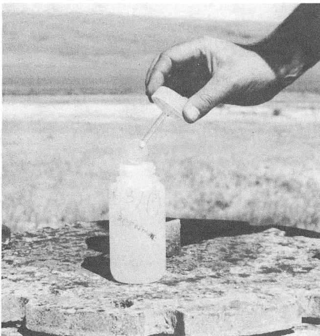
Fig. 1. Method for field monitoring H_2S and sulfide levels in waters. A water sample is placed in the plastic bottle and a silver disk is suspended in the water with a plastic rod attached to the bottle cap. (CBB 748-5750)
