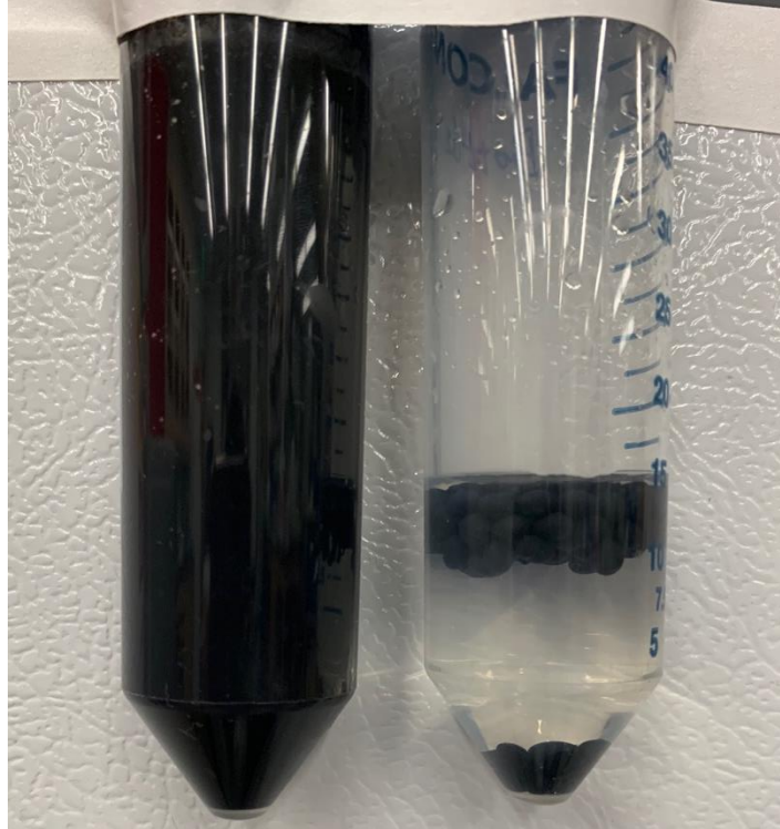
Figure 4.41. Morphological changes of beads in liquids before (right) and after (left) reaction.
