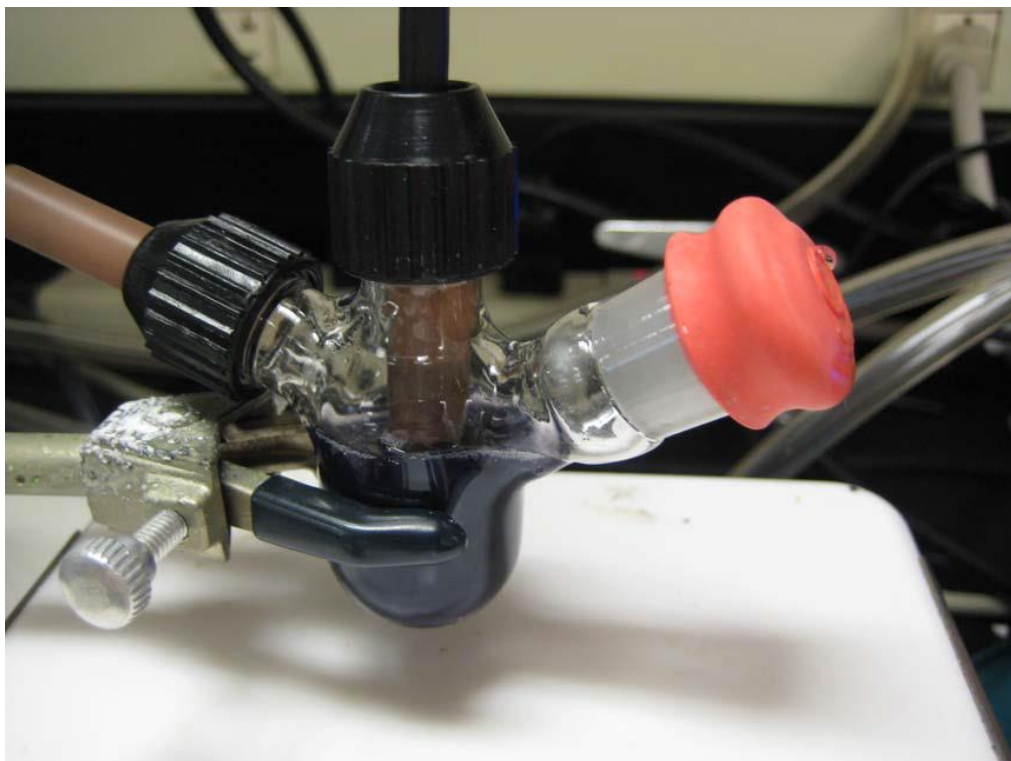
Figure III.2.12. Custom made reaction cell for measuring oxygen levels (Randy Hansen at SC Glass Tech.). A Clark electrode is submerged in reaction mixture and another electrode from the side measures the headspace. The catalyst solution is injected through septum and puncture sealed with grease. Image from ref. 27
