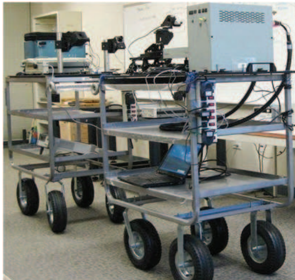
Figure 2.1: The UV testbed (Left cart: photodetector and oscilloscope; right cart: LED/laser transmitter).
