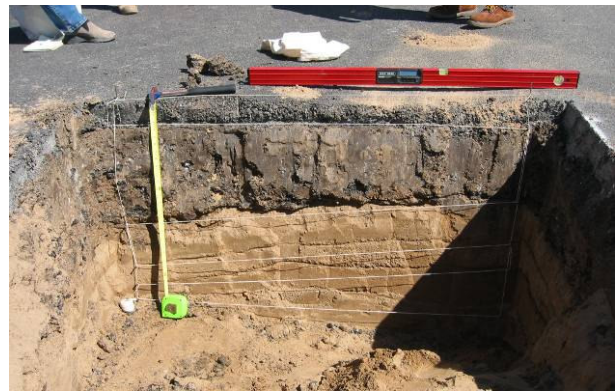
Note variable thickness of all layers.
