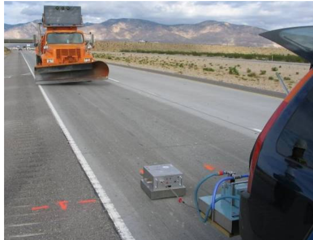
Site selection based on skid resistance (Dynamic friction tester)
