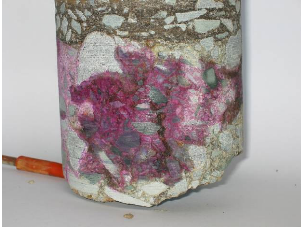
Phenolphthalein reaction on core
