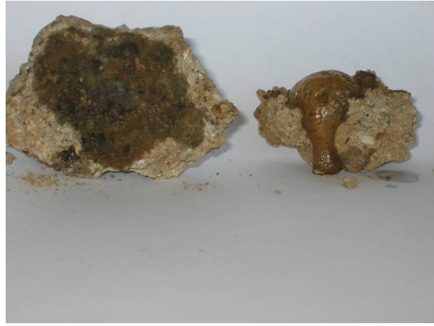
Hydrochloric acid reaction on disintegrated core
