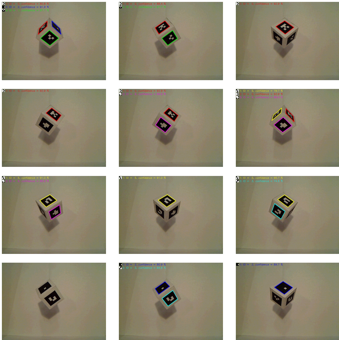
Figure D.7: Cube tracking. The top left corner of each image shows the pattern detected and the detection confidence.
