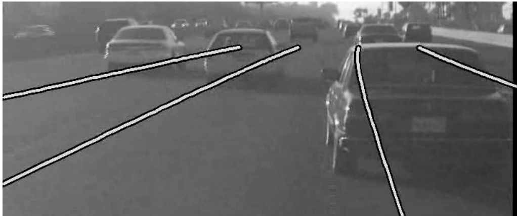
Figure II.17: Error due to occlusion of the road by a vehicle on the dusk dataset on road segment C.
