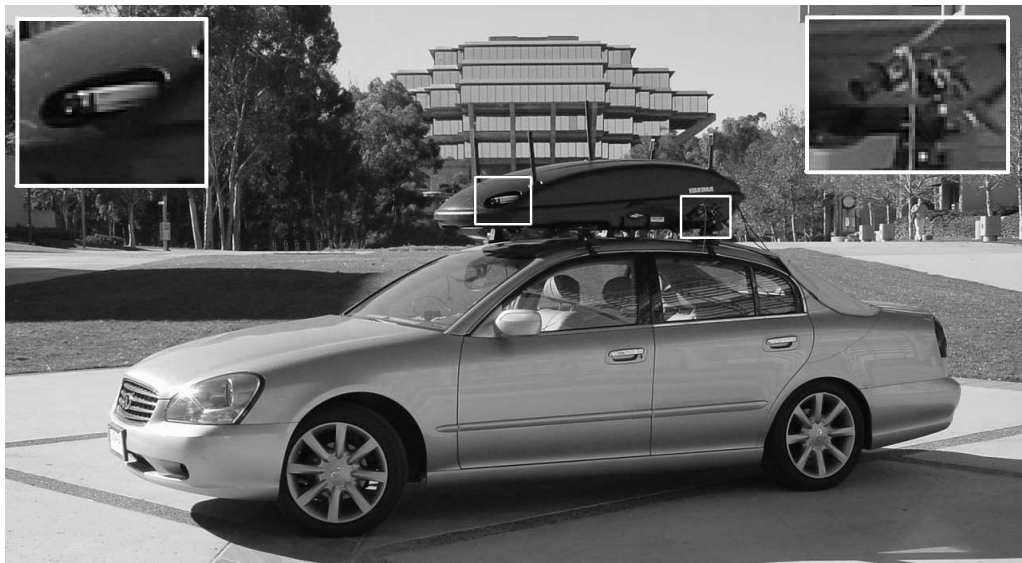
Figure VI.1: The LISA-Q intelligent vehicle test bed. Inset are close up views of the front camera (left inset) used for detection and tracking and side camera (right inset) used for generating ground truth.
