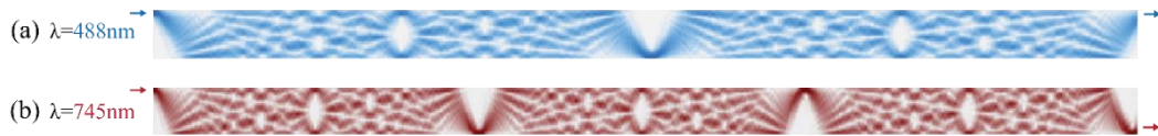
Fig. 5.30 The simulated MMI waveguide patterns on the same device by using a beam propagation method, for two design wavelengths: (a) \lambda_B=488\text{nm} (bar-coupler) and (b) \lambda_C=745\text{nm} (cross-coupler)
