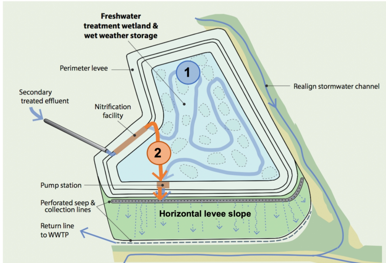
Figure 2-1: The site layout of the experimental horizontal levee test facility (Baye and ESA, 2012). The site included a surface-flow treatment wetland, which doubled as a wet weather equalization basin, a nitrification facility and the horizontal levee slope. The two flow paths correspond to the two flow regimes employed over the monitoring period, in which: (1) nitrified secondary effluent passed through the freshwater treatment wetland prior to being distributed in the horizontal levee slope (blue path) and (2) nitrified secondary effluent bypassed the treatment wetland was fed directly into the horizontal levee slope, in which case a parallel flow of water was also pumped backward through the freshwater treatment wetland (not shown) before returning to the headworks of the wastewater treatment facility (orange path). In both regimes, effluent from the horizontal levee slope was also returned to the headworks of the wastewater treatment plant. A timeline of operational changes is presented in Figure 2-3. The influent sampling location was at the distribution pump preceding the horizontal levee slope.
