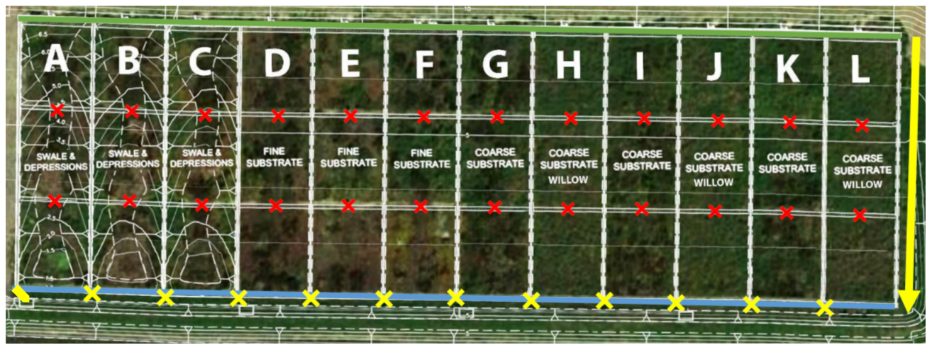
Figure 2-2: Layout of the horizontal levee slope at the test facility showing the individual cells. The four treatments are labeled in the center of each cell. Influent water enters each cell through perforated pipes at the top of the slope represented by the green line. Intermediate wells 15 and 30 m along the slope were located in the center of each cell (denoted by a red X). The effluent was collected in a gravel trench at the end of each slope, represented by the blue line, with effluent sampling ports and flow meters denoted by a yellow X for each cell. The yellow line indicates the direction of flow.
