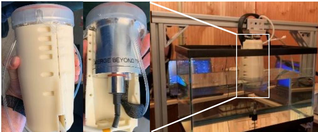
Figure 15: H-102 and cup-shaped mount mounted onto the aluminum frame. Hydrophone was mounted at the bottom of the fish tank.
