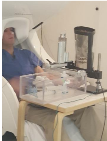
Figure 14: Magnetoencephalography set up with Dr. Lerman sitting in. The transducer was enclosed with cardboard covered by steel foil.
