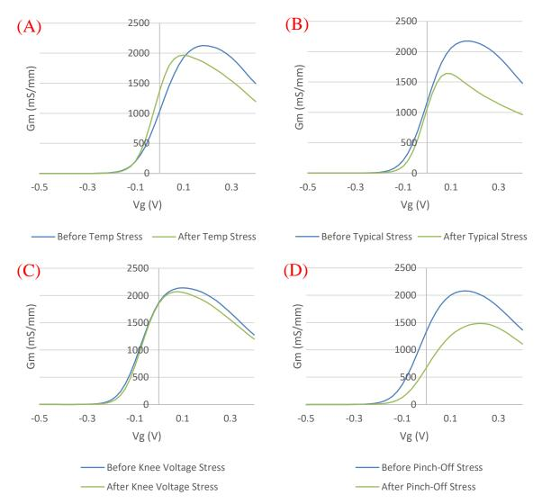
Figure 2.10  $G_m$  at  $V_d$  = 1.0 V before and after (A) temperature, (B) typical operating conditions, (C) knee voltage and (D) pinch-off life tests
