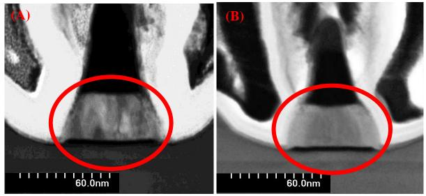
Figure 3.11 (A) STEM image of an unstressed IACC HEMT; (B) STEM image of IACC after pinch-off conditions
