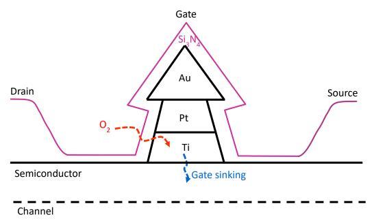
Figure 2.1 Examples of typical III-V failure mechanisms
