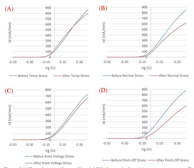
Figure 2.11 Transfer curve  $I_{dmax}$  at  $V_d=1.0~V$  before and after (A) temperature stress, (B) typical operating conditions, (C) knee voltage stress, (D) pinch-off stress
