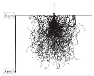
Figure 3.2 SEM interaction volume into a sample surface at a 20 kV accelerating voltage [19]
