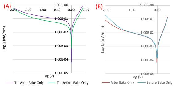
Figure 2.8 (A)  $I_g$ - $V_g$  curve of Ti-metal-gate HEMT before temperature stress and after; (B)  $I_g$ - $V_g$  curve of refractory metal-gate HEMT before temperature stress and after
