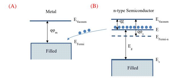
Figure 1.7: (A) Band diagram of a metal; (B) Band diagram of an n-type semiconductor
