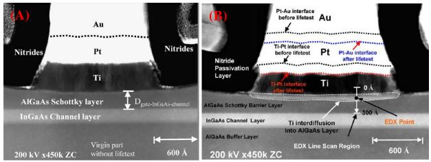
Figure 2.3 STEM image of 0.15 um InP HEMT (A) unstressed, (B) with Pt diffusion at Tchannel 235°C for 96 hours [14]
