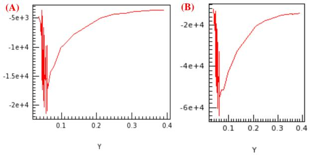
Figure 5.8 Electric-field distribution through the gate at (A) pinch-off stress; (B) knee voltage stress
