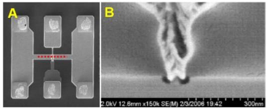
Figure 1.2: (A) Top view SEM image of InP HEMT. The red dotted line indicates the location of the cross-section. (B) Cross-section of a 35 nm InP HEMT
