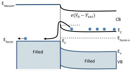
Figure 1.10: Band diagram of Schottky junction under forward bias
