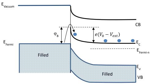
Figure 1.11: Band diagram of Schottky junction under reverse bias
