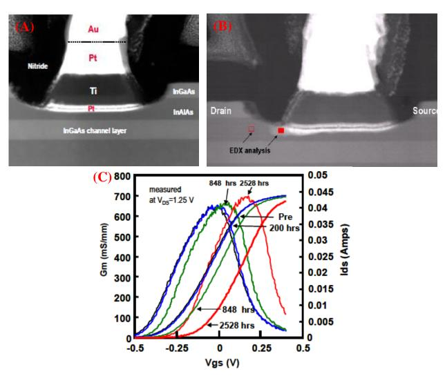
Figure 2.4 STEM image of 0.1 um InP HEMT (A) unstressed, (B) with Pt diffusion at Tchannel 220°C for 2528 hours, (C) positive shift in Gm and Vth [9]
