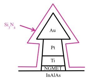
Figure 1.4: Schematic diagram of a cross-section of Schottky gate
