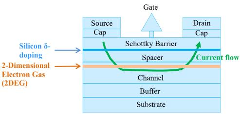
Figure 1.5: Cross-section of a HEMT structure and layers
