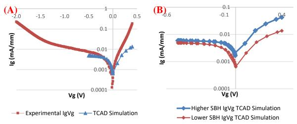
Figure 5.6 (A) IgVg of unstressed device against TCAD simulation; (B) IgVg curve of TCAD simulation with Schottky barrier change
