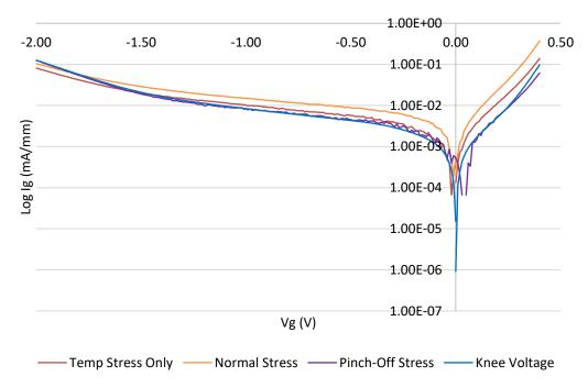
Figure 2.9  $I_g$ - $V_g$  curves of refractory metal-gate HEMT after temperature (blue), typical (pink), pinch-off (orange) and knee voltage stress (brown)
