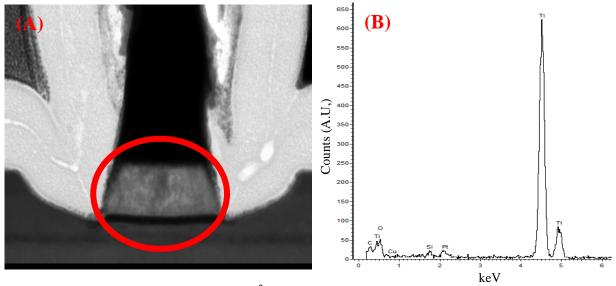
Figure 4.2 (A) STEM image of 1000 Å  $Si_3N_4$  device after a high electric field life test; (B) EDS spectrum of the outer edge of the titanium metal showing less concentration of oxygen
