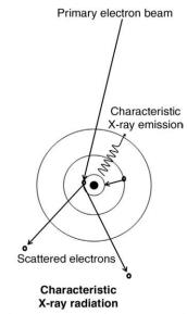
Figure 3.9 Schematic diagram of characteristic X-ray radiation
