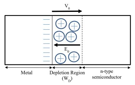
Figure 1.9 Schematic of how the contact potential is formed as the metal and semiconductor come together
