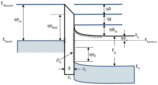
Figure 1.12: Energy band diagram of metal-semiconductor contact with an interfacial layer (vacuum) on the order of atomic distances
