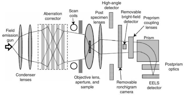
Figure 3.6 Schematic diagram of a STEM
