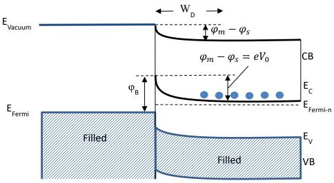
Figure 1.8 Schottky junction band diagram showing the upward band bending of the semiconductor as the materials come into contact
