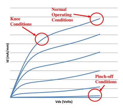
Figure 2.2 I<sub>d</sub>-V<sub>d</sub> curve showing the operating conditions for the accelerated life tests
