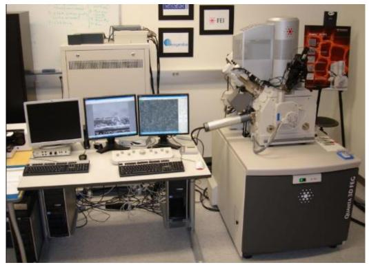
Figure 3.3 FEI Quanta 3D FEG SEM/FIB of IMRI
