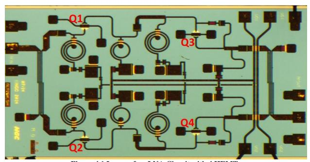
Figure 4.1 Image of an LNA Circuit with 4 HEMTs
