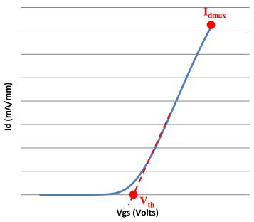
Figure 2.6 Source-to-drain current versus gate-to-source voltage plot determining threshold voltage ( $V_{th}$ ), maximum drain current ( $I_{dmax}$ );  $I_d$  at  $V_d$  = 0.5 V
