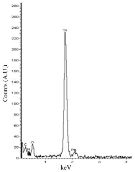
Figure 3.13 EDS spectrum of  $Si_3N_4$  with oxygen diffusing through the passivation layer
