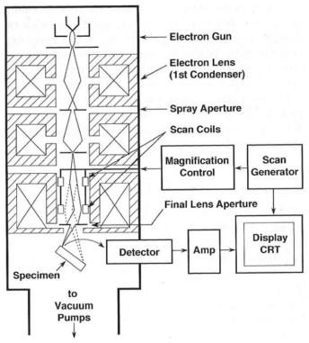
Figure 3.1 SEM schematic drawing
