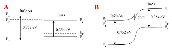
Figure 1.6: (A) Diagram of the band structures of InGaAs and InAs at equilibrium; (B) Semiconductors in contact at equilibrium. A 2DEG is formed at the interface
