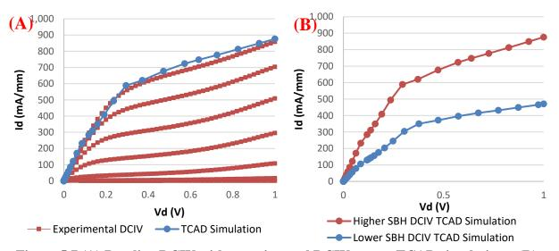
Figure 5.7 (A) Baseline DCIV with experimental DCIV versus TCAD simulations; (B) DCIV Schottky barrier change
