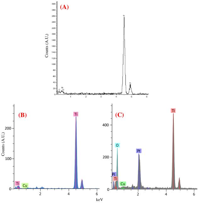
Figure 3.12 EDS spectrum of the (A) outer edge of titanium in unstressed device (B) inner and (C) outer titanium gate metal
