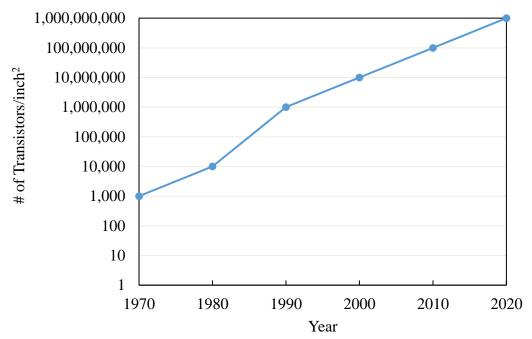
Figure 1.1: Moore's Law: extrapolation of number of transistors placed on a circuit over time [3]
