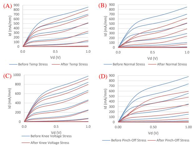
Figure 2.12 DCIV curves before and after (A) temperature, (B) typical operating conditions, (C) knee voltage and (D) pinch-off stresses
