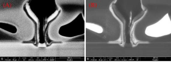
Figure 3.7 (A) Examples of a STEM-HAADF image and (B) STEM-BF image
