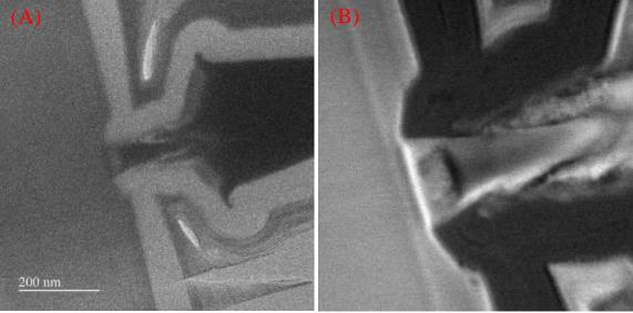
Figure 3.8 (A) STEM image of HEMT gate after nanomilling once; (B) STEM image of HEMT gate after nanomilling twice
